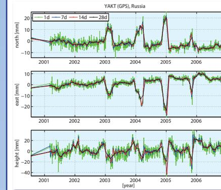
As an example, Fig. 6 shows the residual motions for the GNSS station Yakutsk (YAKT), Russia. In total, four different time series are displayed: the daily GPS-only residuals and the three combined ERF residuals (7d, 14d, 28d).
