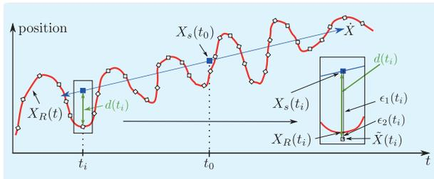
Fig. 3: Station motion parameterization of a secular (blue, continuous linear) and an epoch reference frame (white boxes, discrete). The red line represents the regularized motion of a station position, which is already corrected for conventional models (e.g., Earth tides, ocean tide loading, ...).
