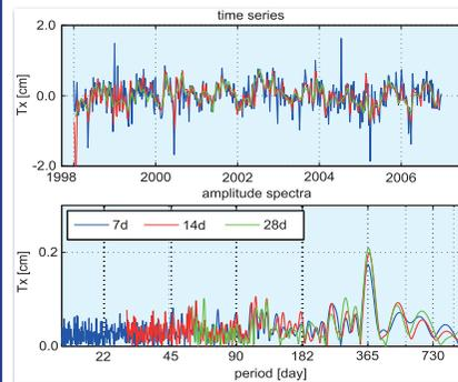
Fig. 5: Time series and spectra of the x-translations for selected GNSS stations of the combined ERFs w.r.t. the combined MRF.
