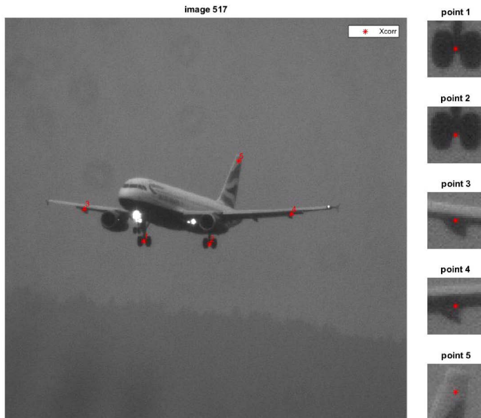
Figure 4.91: Aircraft tracked and measured at Zürich airport by a QDaedalus system.
