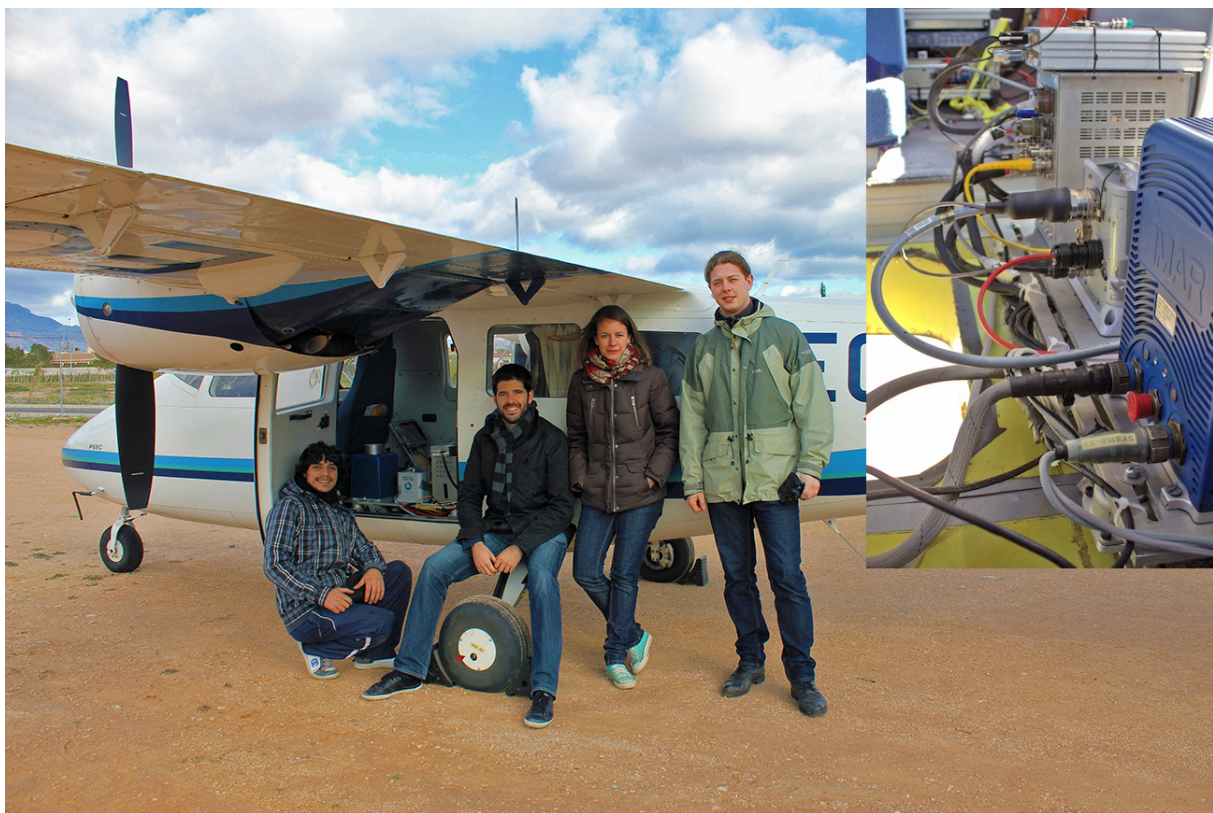
Figure 2.38: Kinematic airborne gravity sensor (two navigation-grade strapdown inertial sensors with geodetic-grade GNSS receivers) mounted in the plane.
