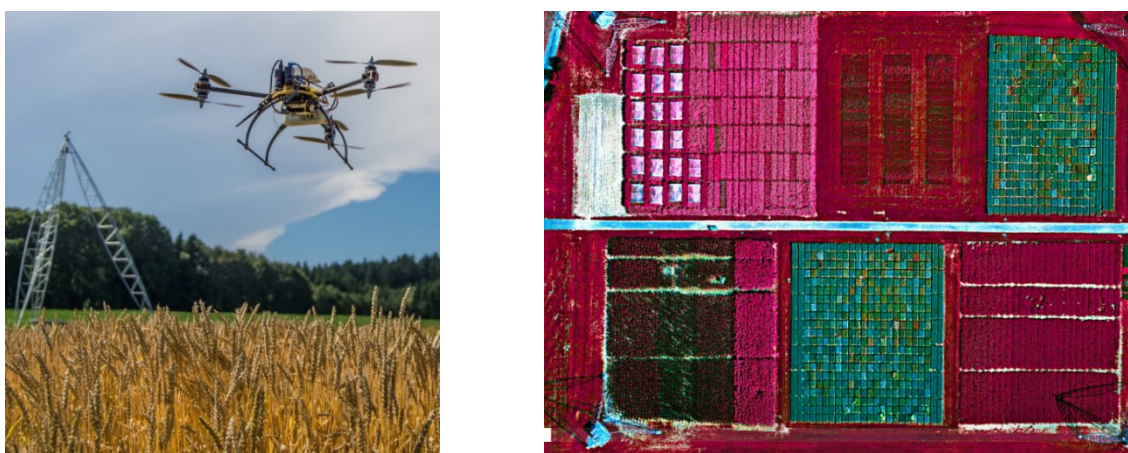
Figure 4.19: HSI mapping with the help of UAV on crop field (left); mapping of phenotypes based on HIS (right)
