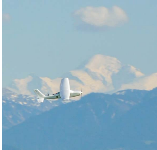
Figure 4.2: Fixed-wing micro UAV platform in a mapping flight with precise orientation sensors.
