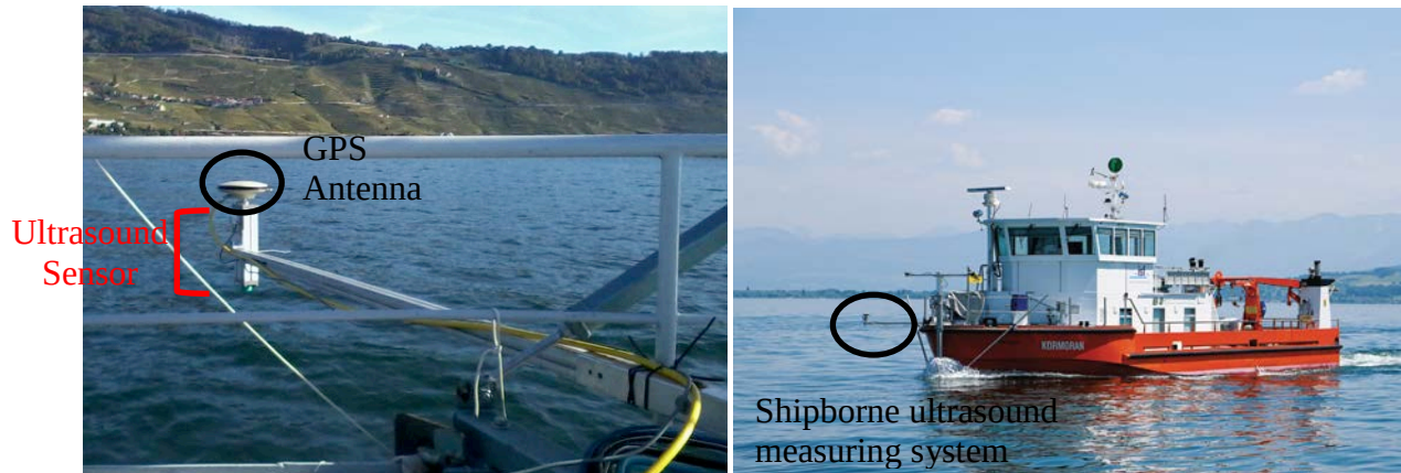
Figure 2.27: Shipborne ultrasound altimetry measuring the Lake Geneva (left)(credits: Institut F.-A. Forel, Uni Genève) and Lake Constance (right) on the survey vessel “Kormoran” of the Institut für Seenforschung (credits: “Tiefenschärfe hochauflösende Vermessung des Bodensees”).
