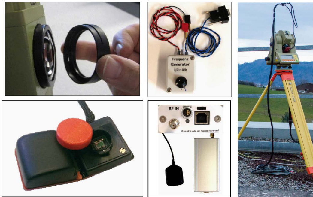
Figure 4.85: Main hardware components of the QDaedalus system.
